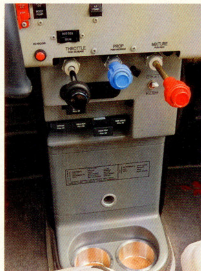
A Garmin G1000 integrated flight display system comes standard (top). The G1000 makes a clean, professional-looking panel. Vernier-type engine controls make for precise inputs (above). Of course, no new airplane would be complete without cup holders.
